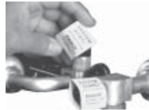
Slide over charge port cap
