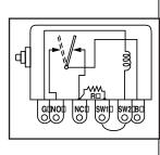
**518APH** Allows for SWICHGAGE<sup>®</sup> and/or N.C. contacts to be wired "Closed Loop" (in series). Any contact open or SWICHGAGE<sup>®</sup> contact close in the circuit shunt trips the 518APH. Specify 12 or 24 VDC. Contacts 10 amps 24V. 14 amp fuse.
