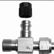
Standard Flow R-134a O-Ring Fitting w/o Service Ports on compressor
