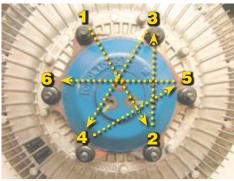
Figure 3 Torque sequence
